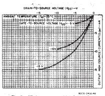
Flg. 8 – Minimum output high (source) current characteristics.
