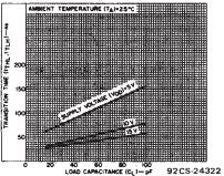
Fig. 9 – Typical transition time vs. load capacitance.
