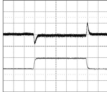
Conditions: Input Voltage = 24 VDC Output Current = 5 to 10 A Bandwidth Limit = 20 MHz Traces: Bottom Trace: Output current A/div = 5 A Top Trace: Output voltage response V/div = 100 mV Horizontal Resolution = 200 \mu s/div
