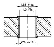
Drill hole specification for chemical surfaces (Ni/Au)
