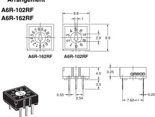
Side-actuated Flat Models with 4×1 Terminal Arrangement
