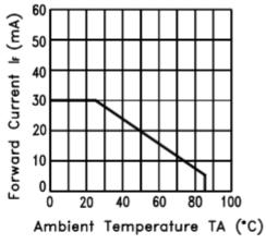
Fig.3 FORWARD CURRENT DERATING CURVE
