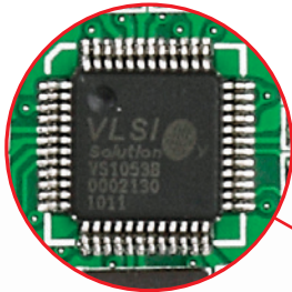
Figure 8-1: On-board VS1053 MP3 codec
