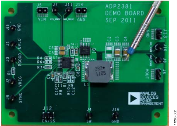
Figure 2. Measuring Output Voltage Ripple
