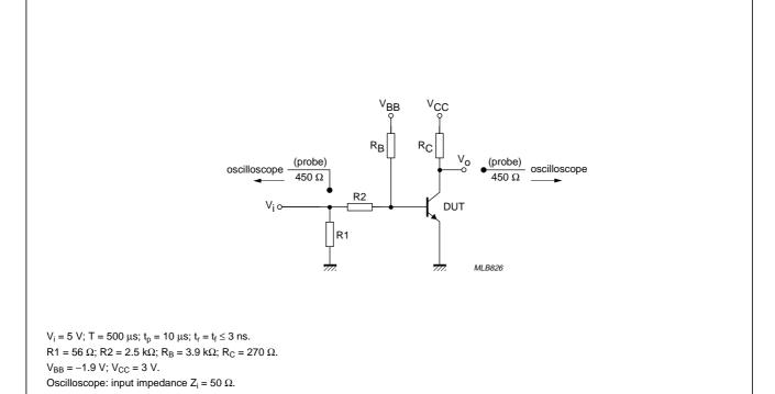
Fig.7 Test circuit for switching times.
