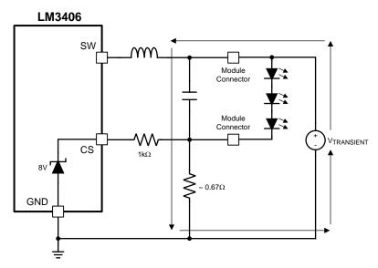
CS Pin, Transient Path with Protection
