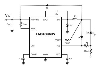
Two Methods of Output Open Circuit Protection
