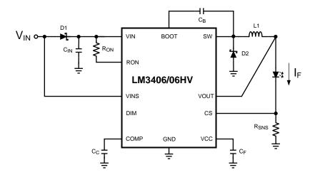
Typical Application using Two-Wire Dimming
