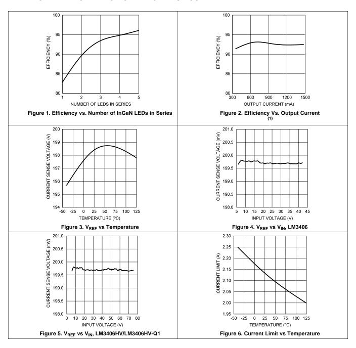
V<sub>IN</sub> = 24V, I<sub>F</sub> = 1A, T<sub>A</sub> = 25°C, and the load consists of three InGaN LEDs in series unless otherwise noted. See the Bill of Materials table at the end of the datasheet.
