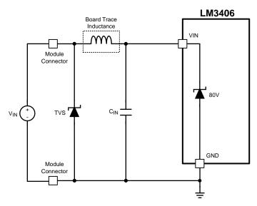
**VIN Pin with Typical Input Protection**
