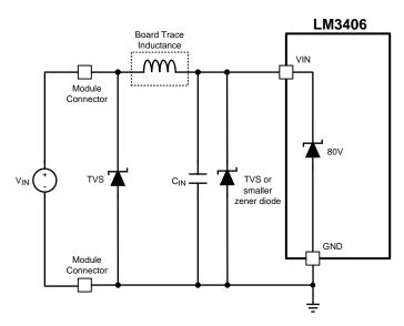
**VIN Pin with Additional Input Protection**
