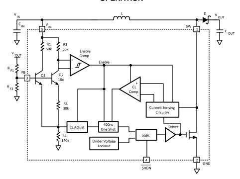
Figure 15. LM2703 Block Diagram
