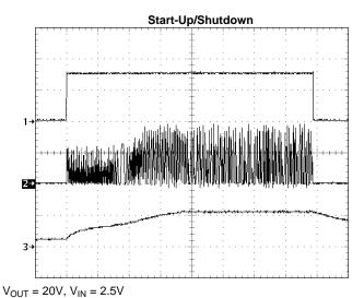
$V_{OUT} = 20V$ ,  $V_{IN} = 2.5V$ 1) Load, 1mA to 10mA to 1mA, DC
