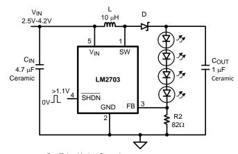
C<sub>IN</sub>: Taiyo Yuden Ceramic C<sub>OUT</sub>: Taiyo Yuden Ceramic L: Coilcraft DT1608C-103 or Murata LQY33PN100M02 (low profile) D: Motorola MBRM130LT3
