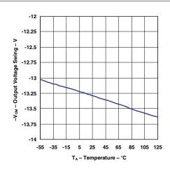
Figure 9. Negative Output Voltage Swing vs Temperature (V<sub>CC</sub> =  $\pm 15$  V, R<sub>L</sub> = 10 k $\Omega$ )
