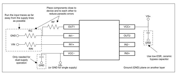
Figure 19. Operational Amplifier Board Layout for Noninverting Configuration
