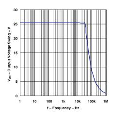
Figure 6. Output Voltage Swing vs Frequency  $(V_{CC} = \pm 15 \text{ V}, R_L = 2 \text{ k}\Omega, T_A = 25^{\circ}\text{C})$
