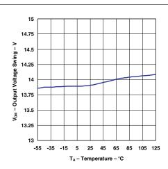
Figure 8. Output Voltage Swing vs Temperature ( $V_{CC} = \pm 15 \text{ V}, R_L = 10 \text{ k}\Omega$ )
