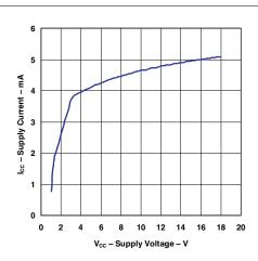
Figure 1. Supply Current vs Supply Voltage  $(T_A = 25^{\circ}C)$
