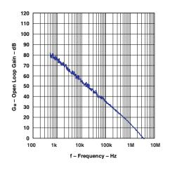
Figure 10. Open Loop Gain vs Frequency ( $V_{CC}$  = ±15 V,  $R_L$  = 2 k $\Omega$ ,  $C_L$  = 22 pF,  $T_A$  = 25°C)
