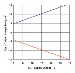
Figure 5. Output Voltage Swing vs Supply Voltage  $(R_L = 2 k\Omega, T_A = 25^{\circ}C)$
