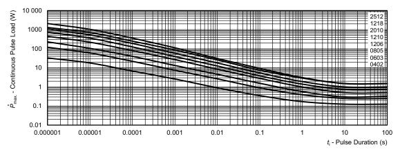
Maximum pulse load, continuous pulses; applicable if  $\bar{P} \leq P \left(\vartheta_{amb}\right)$  and  $\hat{U} \leq \hat{U}_{max}$ ; for permissible resistance change equivalent to 8000 h operation
