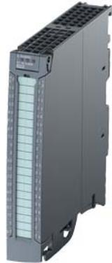
SIMATIC S7-1500 Digital input module, DI 32x24 V DC BA, 32 channels in groups of 16, Input delay typ. 3.2 ms, Input type 3 (IEC 61131); Delivery incl. front connector Push-in
