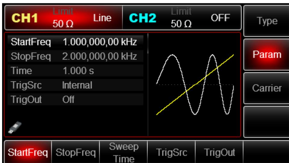
Figure 3 - 33 Set frequency sweep parameters
