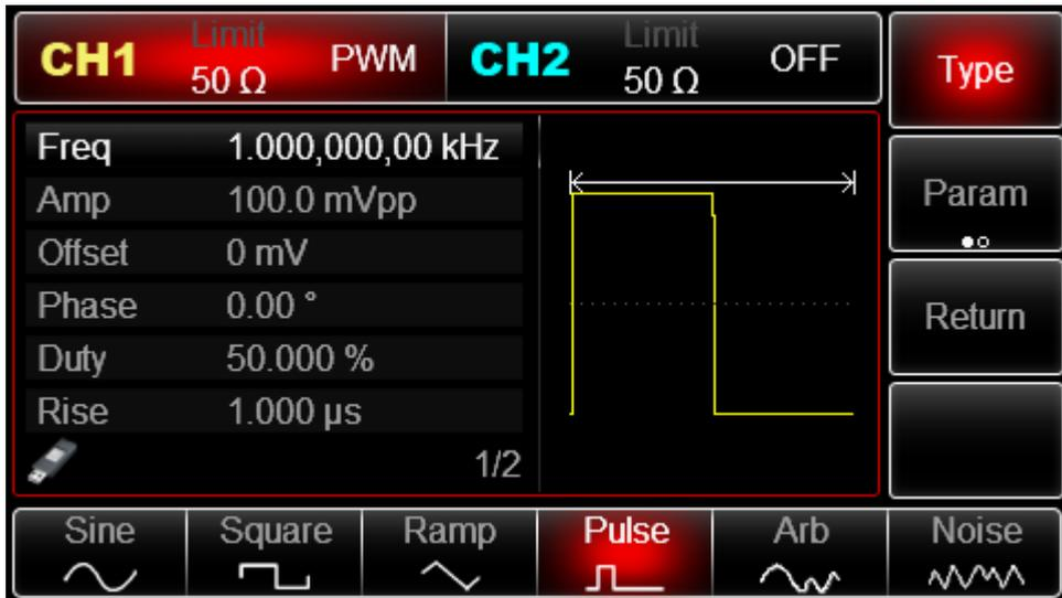
Figure 3 - 21 Set carrier waveform Set carrier frequency
