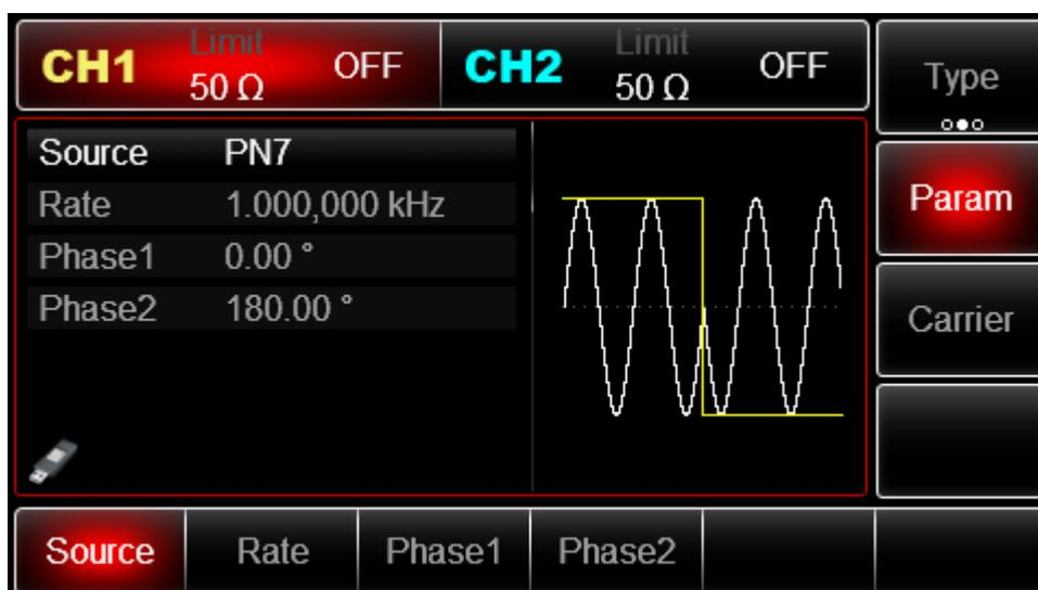
To set some parameter, press corresponding soft key, input the required value and select the unit.
