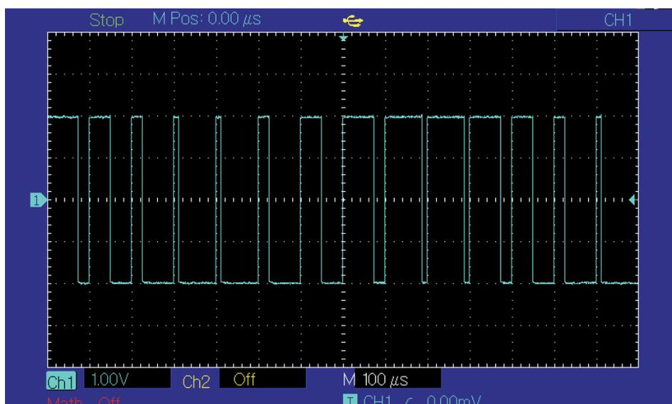
Figure 3 - 30 Observe PWM waveform with oscilloscope
