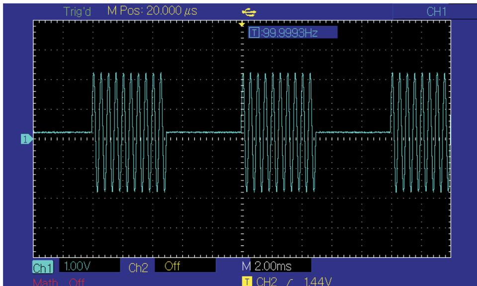
Figure 3 - 4 OSK waveform with oscilloscope
