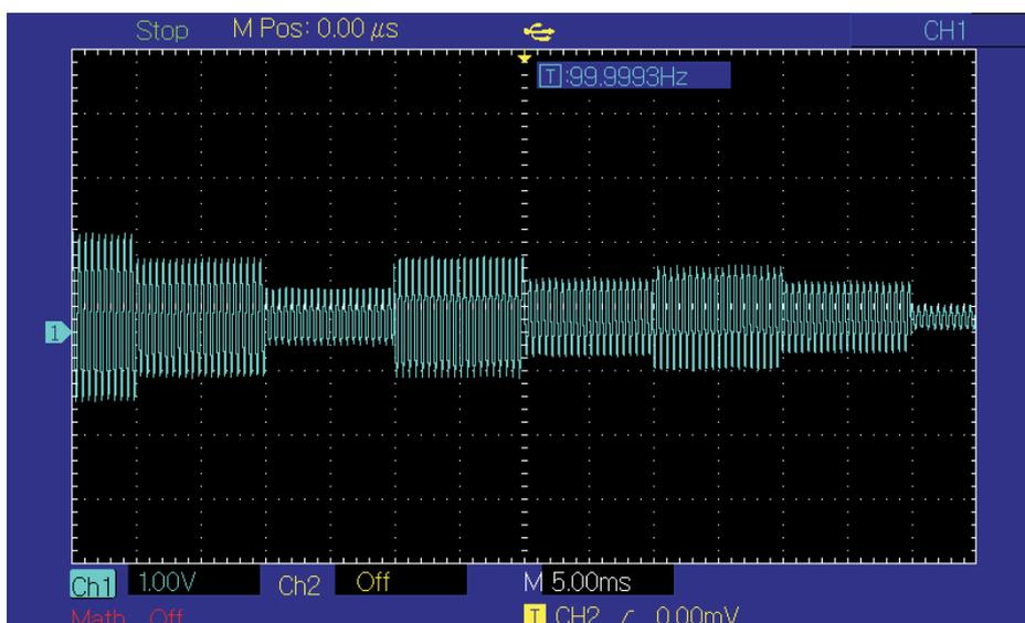
Figure 3 -19 Observe QAM waveform with oscilloscope
