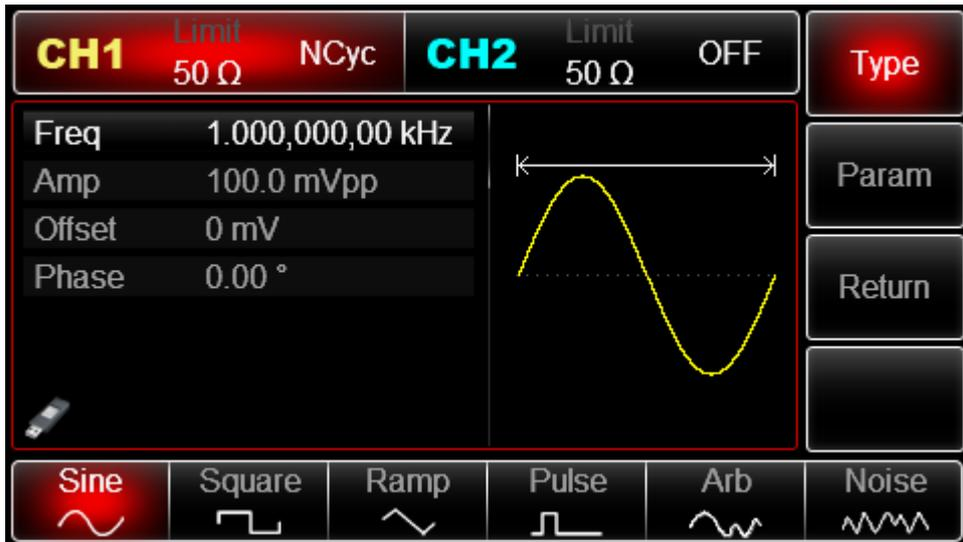
Figure 3 -53 Select waveform of pulse train
