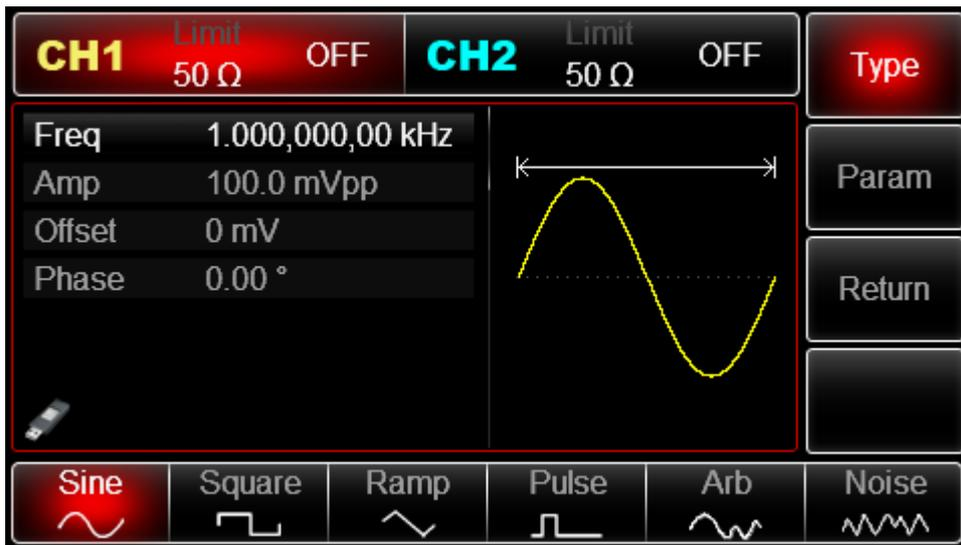
Figure 3 - 1 Select carrier waveform Set carrier frequency
