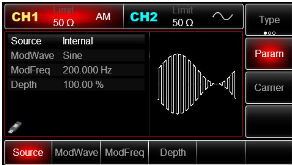
Press **Param** → **depth** soft key again, then enter number 80 and press **%** soft key with number keyboard for setting modulation depth.
