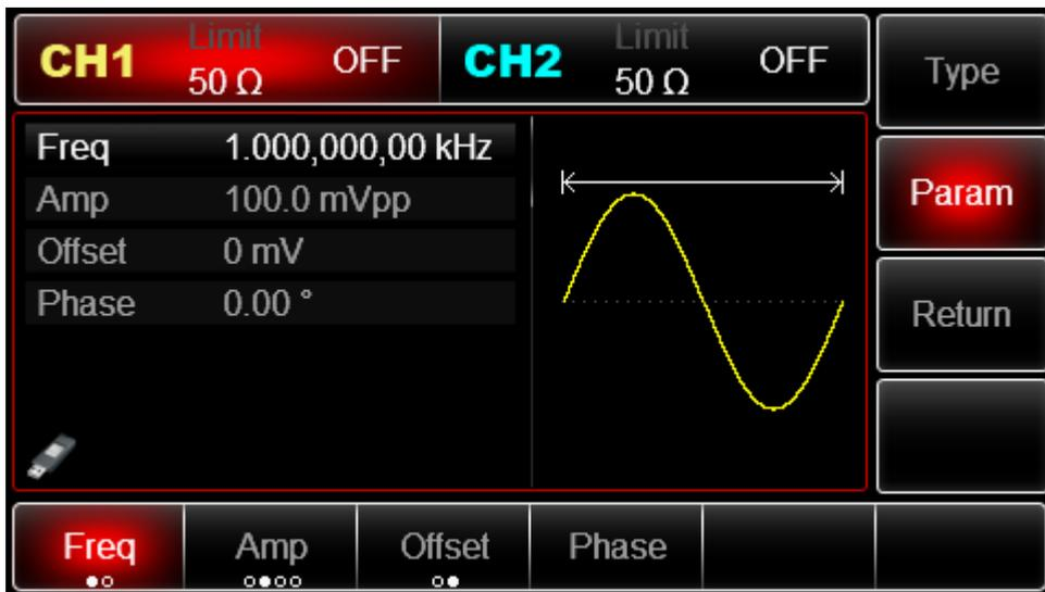
Press corresponding soft key first, then enter required numerical value, and select the unit.
