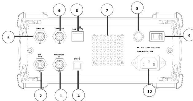
1. External analog modulation input connector
