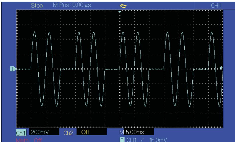
Figure 3 -58 Observe BURST waveform with oscilloscope
