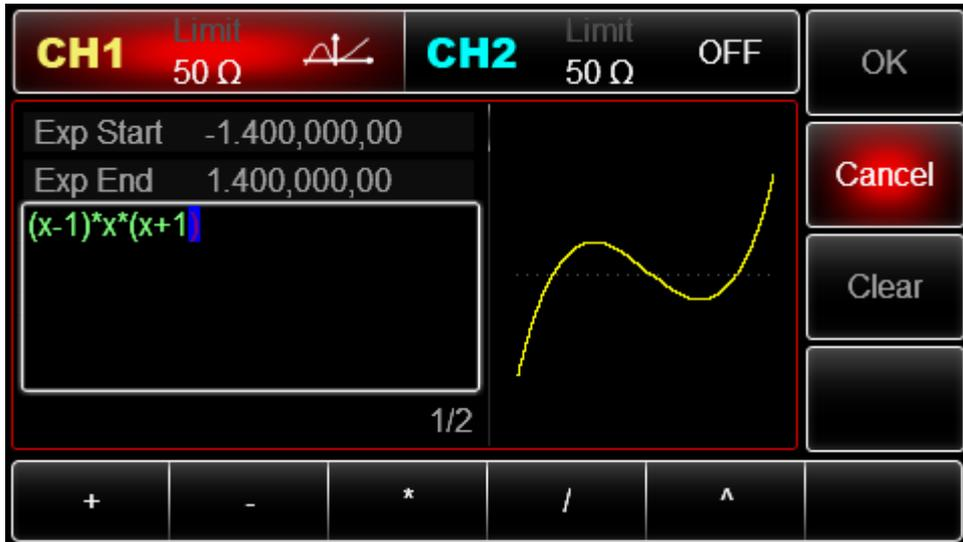
The default initial value is  $0^\circ$ , end value is  $180^\circ$ , and expression is  $\sin(x)$ . The unit can be in rad or  $^\circ$ . The setup procedures are as following:
