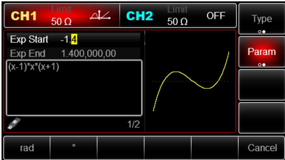
18 types of operational functions are supported in this instrument. Expression enter into the expression editing interface, press Next to cycle switch operational symbol or expression. For example, input  $(x-1)x(x+1)$ , the interface is as below:
