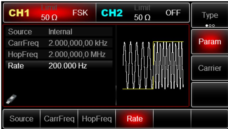
The shape of FSK modulation waveform checked through oscilloscope is shown as following:
