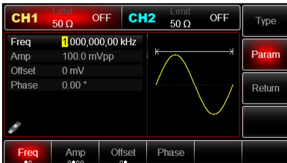
If you need to set up the parameter, input the value and then select the unit.
