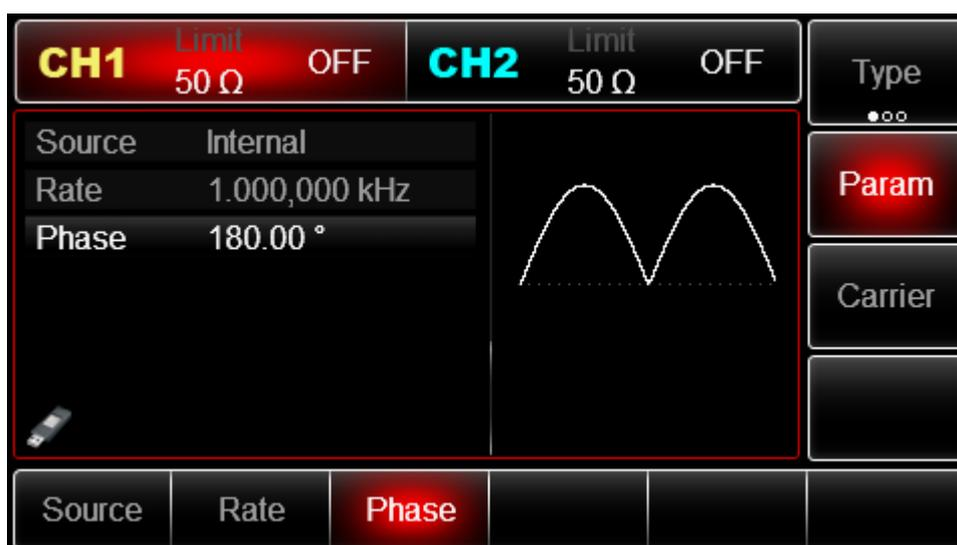
The shape of PSK modulation waveform checked through oscilloscope is shown as following:
