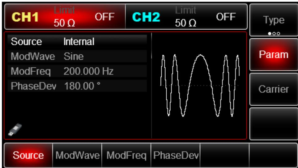
Press **Param** → **PhaseDev** soft key, then enter number 200 and press ° soft key with number keyboard for setting phase deviation.
