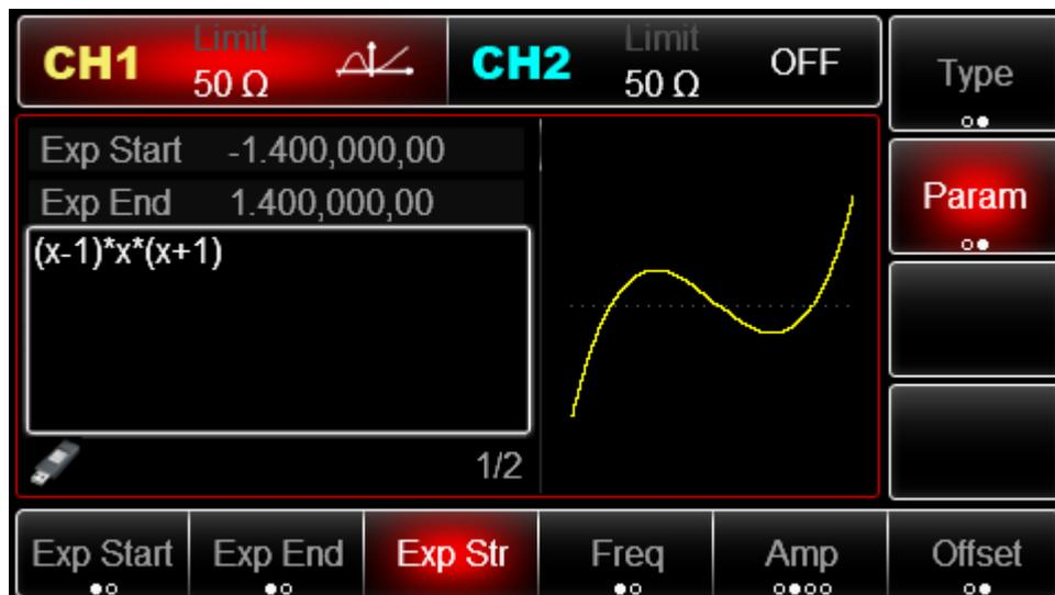
The output from the signal source is duplicate signal within limited period, therefore, it is necessary to define the range of the variable in the expression  $f(x)$ . The range of  $x$  is determined by **Initial value** and **End value**. Press **Initial value** to activate this parameter. Use the keypad to input 1.4rad, the unit can be ° or rad, the interface is as below:
