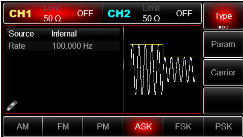
Set Carrier Wave Signal Parameter Press **Carrier** → **Type** → **Sine** in turn
