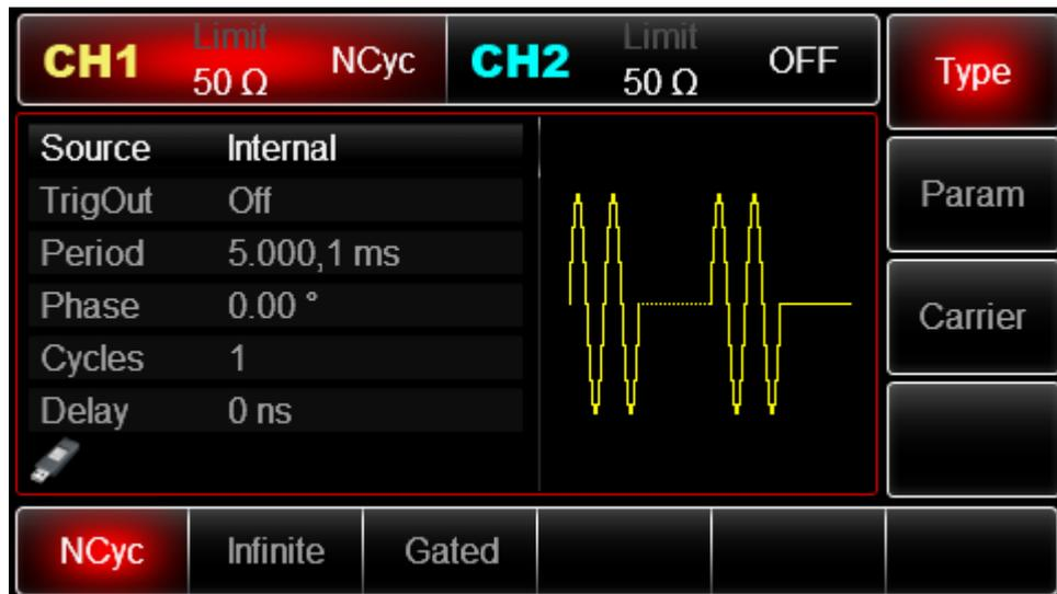
Figure 3 - 55 Set pulse train parameters
