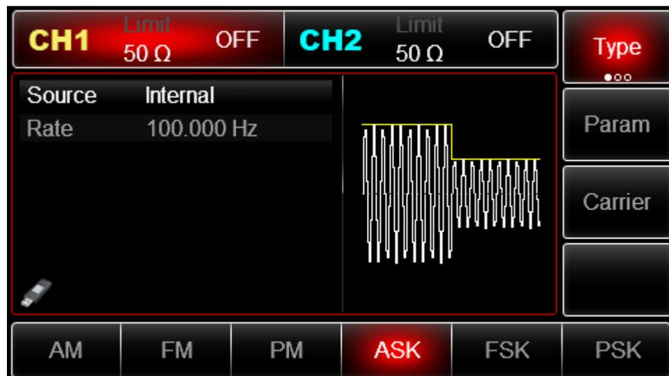
Press **Param** → **Rate** soft key again, then enter number 300 and press **Hz** soft key with number keyboard for setting ASK rate.
