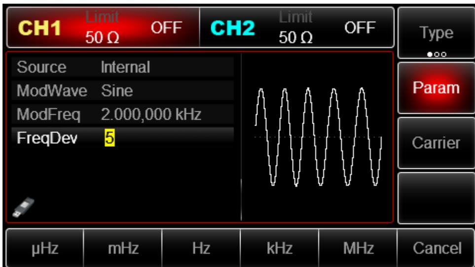
Press **CH1** button start channel 1 output quickly. Or enable output by pressing **Utility** and then **CH1 Setting**. After channel output is opened, backlight of **CH1** button is on, and on the right side of channel information label, the font “OFF” changes to “FM”, meaning open channel 1 output.
