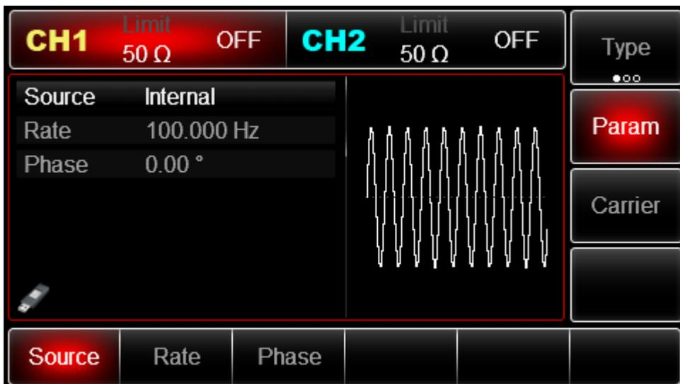
Press corresponding soft key, then enter required numerical value, and select the unit.
