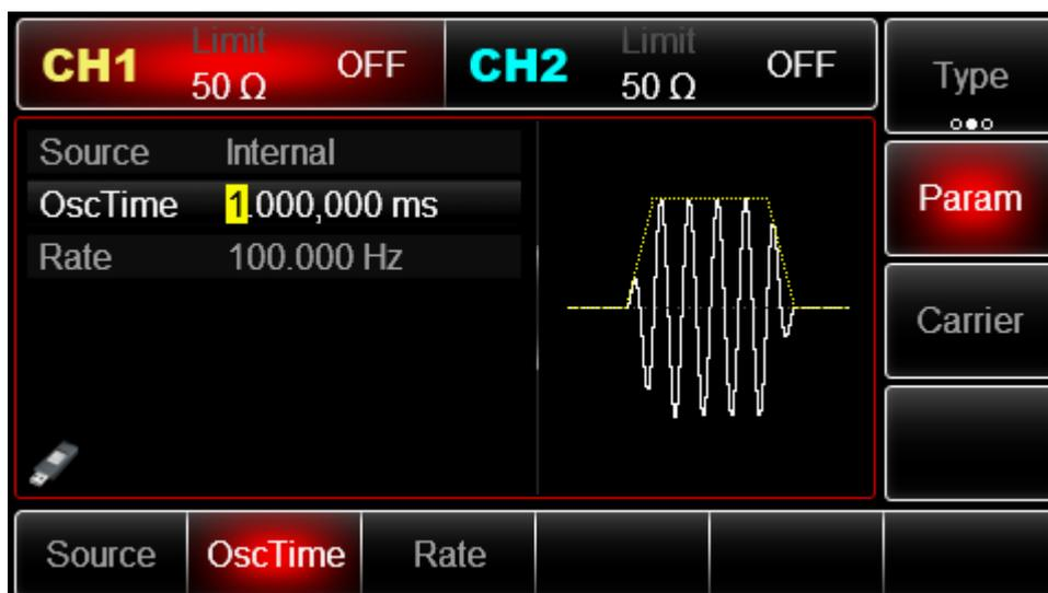
You can set with multi-functional knob and direction key directly on this interface. You can also press corresponding soft keys of function again, when the interface below will pop up. To set some parameter, press corresponding soft key, input the required value and select the unit.
