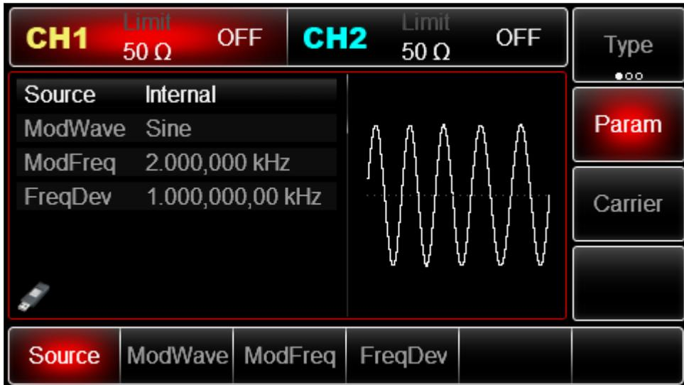
Press **Param** → **FreDev** soft key, then enter number 5 and press **kHz** soft key with number keyboard for setting frequency deviation.
