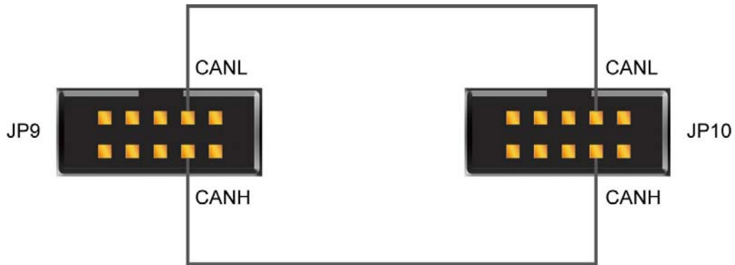
Figure 5-7 Wiring for CAN loopback test
