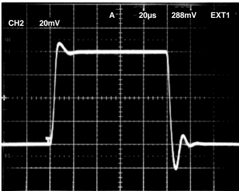
Figure 25. Small Signal Pulse Response, G = +5, R_L = 20 k\Omega, C_L = 50 pF
