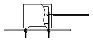
Temperature monitored inside the capacitor.
