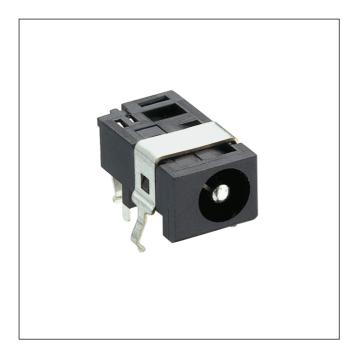
Power supply chassis socket acc. to JEITA RC-5320A JSAJ21, angular version, with break contact, for printed circuit boards
