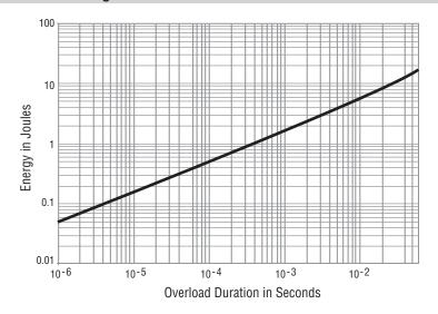
The energy absorbed by the resistor expressed in Joules can be calculated by multiplying the peak power of the pulse in watts times the length of the pulse in seconds.
