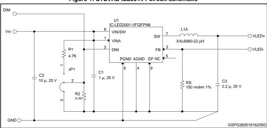
Figure 1: STEVAL-ILL054V1 circuit schematic
