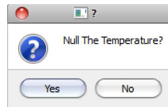
FIGURE 10. INPUT BOX THAT APPEARS WHEN ENABLING THE EXTERNAL TEMPERATURE SENSOR
