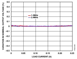
Figure 5. Boost Regulator Load Regulation, Input Supply Voltage Range  $(V_{IN}) = 5 V$ ,  $V_{POS} = 15 V$
