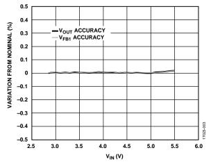
Figure 3. Boost Regulator Line Regulation,  $V_{POS} = 15 \text{ V}$ , Switching Frequency  $(f_{SW}) = 1.2 \text{ MHz}$ , 15 mA Load,  $T_A = 25 ^{\circ}\text{C}$
