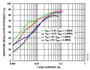
Figure 8. Inverting Regulator Efficiency vs. Load Current,  $V_{NEG} = -15 V$ ,  $T_A = 25 ^{\circ} C$
