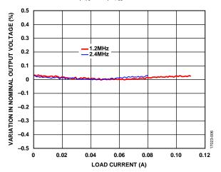
Figure 6. Inverting Regulator Load Regulation,  $V_{IN} = 5 V$ ,  $V_{NEG} = -15 V$
