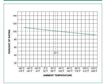
1. Rerating depicted in this curve is in addition to the standard derating of 25% for continuous operation.
