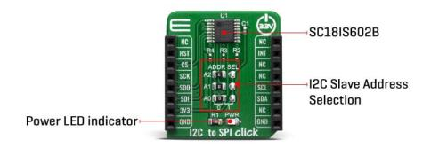
The I2C to SPi Click provides a byte-oriented I2C-bus interface that supports data transfers up to 400 kHz. When the I2C-bus master is reading data from the click board™, the device will be a slave-transmitter. It also can be a slave-receiver when the I2C-bus master is sending data. The SC18IS602B acts as an I2C-bus master at no time. However, it does have the ability to hold the SCL line LOW between bytes to complete its internal processes.
