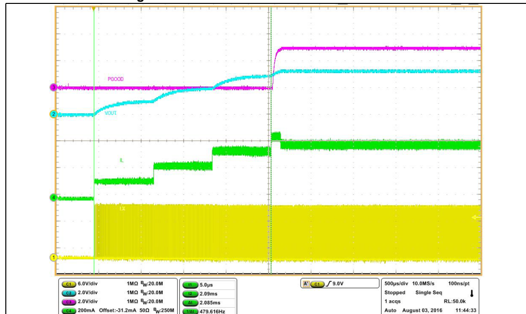
Figure 18. Soft-start feature with resistive load
