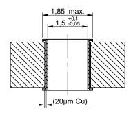
Drill hole specification for chemical surfaces (Ni/Au)
