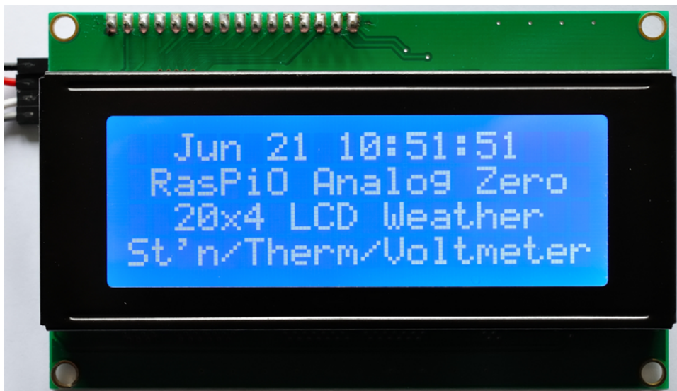
Demo script showing 20x4 LCD clock
