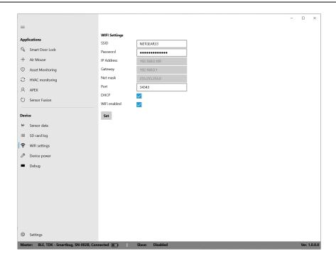
Once the **Set** button is pressed, the device will disconnect the BLE and initiate the WiFi connection to the specified router. The BLE link status will change to **Disconnected** and the module's blue LEDs will turn off and the green LED on the Add-On board will blink. This means the device is now connected to the WiFi router and is ready to communicate through a TCP socket.
