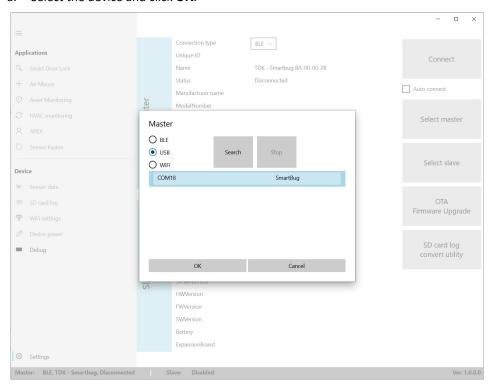
When USB device is selected, press the **Connect** button to connect the SmartBug module to the SmartBug App. After clicking connect, wait a few seconds until the Master device parameters appear. If the **Auto connect** checkbox is checked, the selected device will connect automatically on the application restart.
