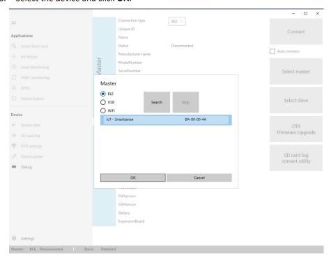
When the BLE device is selected, press the **Connect** button to connect the SmartBug module to the SmartBug App. After clicking connect, wait a few seconds until the Master device parameters appear. If the **Auto connect** checkbox is checked, the selected device will connect automatically on the application restart.
