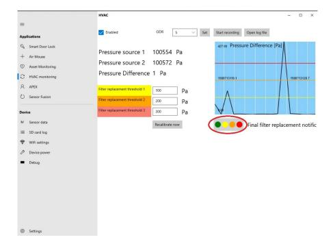
6. Record the differential pressure log along with absolute pressure sensor readings.
