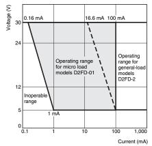
However, even when using microload models within the operating range shown above, if inrush current or inductive voltage spikes occur when the contact is opened or closed, it may increase contact wear and so decrease the service life. Therefore, insert a contact protection circuit where necessary.
