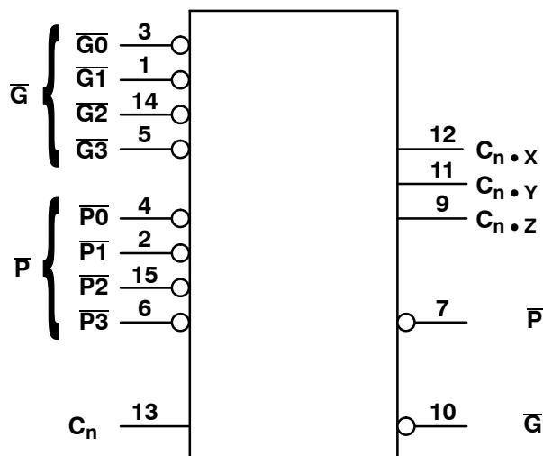
$V_{DD} = \text{Pin 16}$
