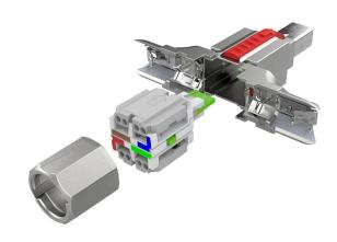
TE Connectivity (TE) Industrial Mini I/O connector can be used in Cat6A Ethernet connections where fast and flawless field installation is an important requirement. It can be connected to the cable without special tools and can accommodate 8-wire AWG24/26 cables.
