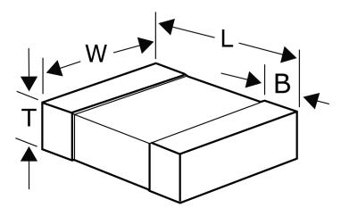
**General Information** Series VC Type Varistors Style SMD Chip Description Surface Mount Varistors Features Low Voltage Termination Nickel Tin RoHS Yes Qualifications IEC, UL, AEC-Q200 AEC-Q200 Yes
