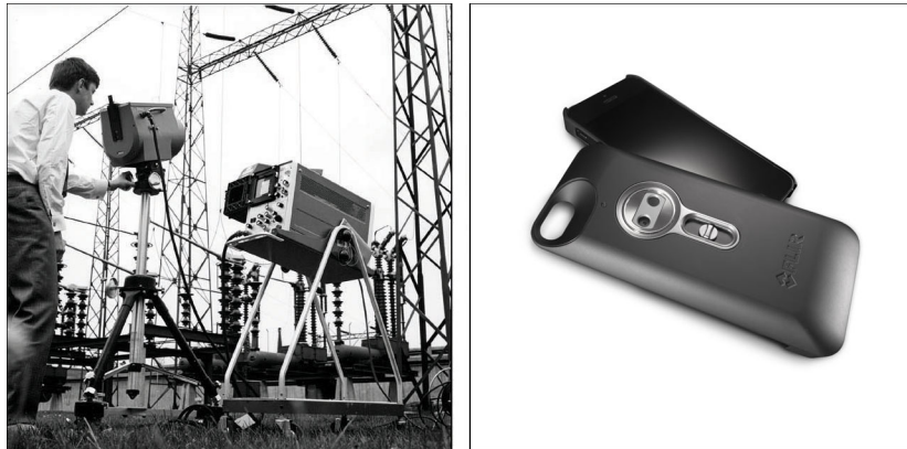
Figure 23.2 LEFT: Thermovision Model 661 from 1969. The camera weighed approximately 25 kg (55 lb.), the oscilloscope 20 kg (44 lb.), and the tripod 15 kg (33 lb.). The operator also needed a 220 VAC generator set, and a 10 L (2.6 US gallon) jar with liquid nitrogen. To the left of the oscilloscope the Polaroid attachment (6 kg/13 lb.) can be seen. RIGHT: FLIR One, which was launched in January 2014, is a slide-on attachment that gives iPhones thermal imaging capabilities. Weight: 90 g (3.2 oz.).
