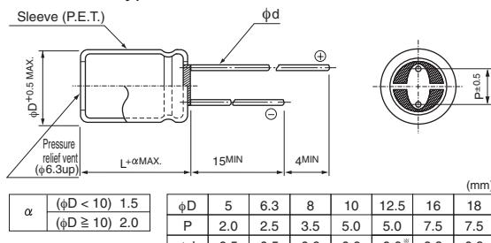
\*In case  $L > 25$  for the  $\phi 12.5$  dia. unit, lead dia.  $\phi d = 0.8\text{mm}$
