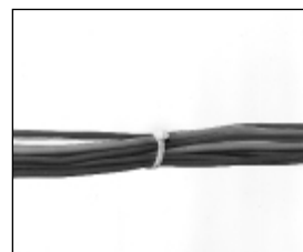
4. Finished tie holds cables firmly.
