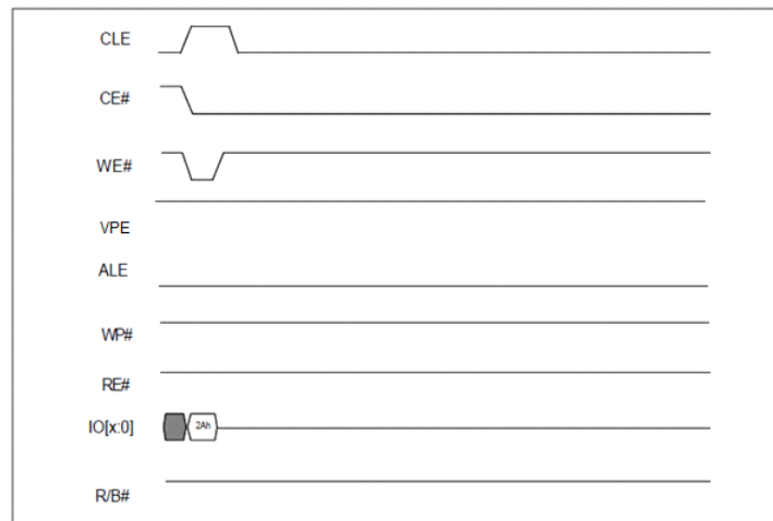
Figure 8. Waveforms for the Lock-down Command
