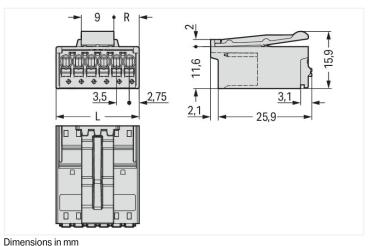
L = (pole no. x pin spacing) + 2 mm Even pole number R = (L – 9 mm) : 2 Odd pole number R = (L – 12.5 mm) : 2
