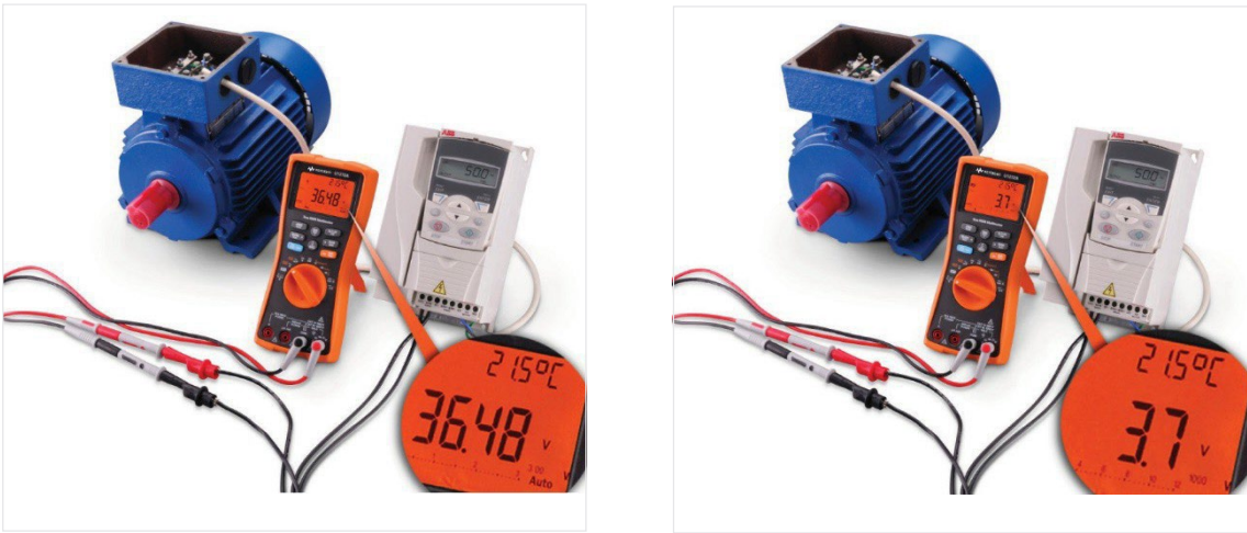
Figure 2. U1272A helps you identify the presence of stray voltage on a disconnected wire running parallel with the wire powering up the VFD to an industrial motor. The image on the right shows the U1272A in low impedance mode.
