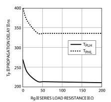
Figure 17: Transfer Characteristics
