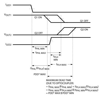
\*PDD = PROPAGATION DELAY DIFFERENCE NOTE: FOR DEAD TIME AND PDD CALCULATIONS, ALL PROPAGATION DELAYS ARE TAKEN AT THE SAME TEMPERATURE AND TEST CONDITIONS.
