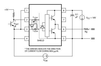
Figure 26: Not Recommended Open Collector Drive Circuit
