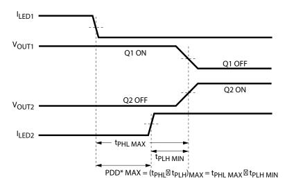
\*PDD = PROPAGATION DELAY DIFFERENCE NOTE: FOR PDD CALCULATIONS, THE PROPAGATION DELAYS ARE TAKEN AT THE SAME TEMPERATURE AND TEST CONDITIONS.
