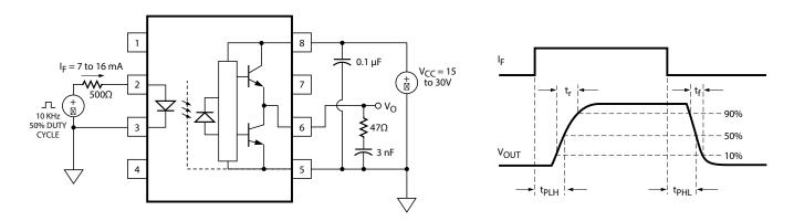
Figure 20: CMR Test Circuit and Waveforms
