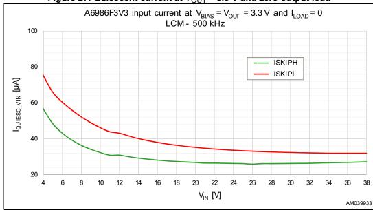
Figure 27. Quiescent current at  $V_{OUT}$  = 3.3 V and zero output load
