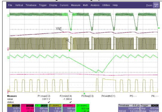
Figure 35. Overvoltage operation
