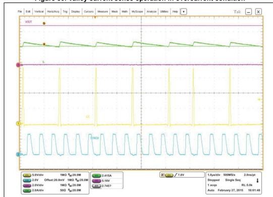
Figure 30. Valley current sense operation in overcurrent condition
