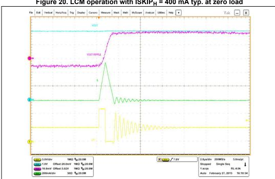
Figure 20. LCM operation with ISKIP<sub>H</sub> = 400 mA typ. at zero load
