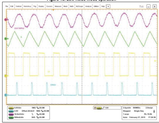
Figure 16. Low noise mode operation
