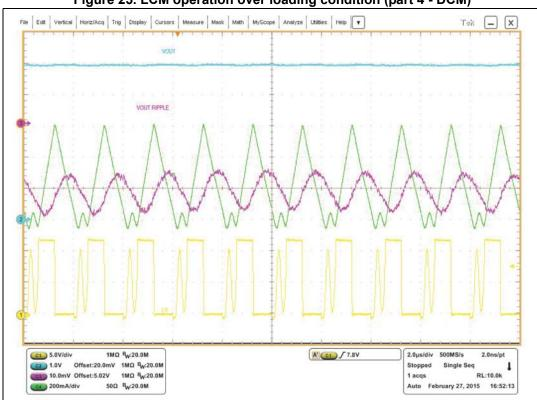
Figure 25. LCM operation over loading condition (part 4 - DCM)
