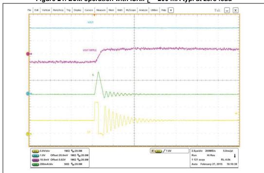
The LCM operation satisfies the requirements of the unswitched car body applications (KL30). These applications are directly connected to the battery and are operating when the engine is disabled. The typical load when the car is parked is represented by a CAN transceiver and a microcontroller in sleep mode (total load is around 20 - 30  $\mu$ A). As soon as the transceiver recognizes a valid word in the bus, it awakes the  $\mu$ C and the rest of the application.
