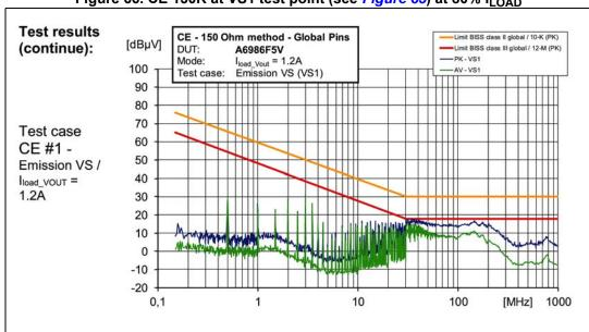
Figure 66. CE 150R at VS1 test point (see Figure 65) at 80% I<sub>LOAD</sub>
