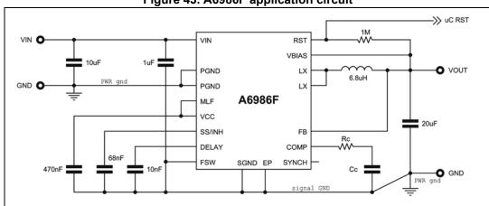
Figure 43. A6986F application circuit
