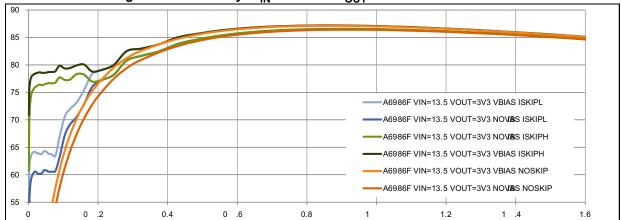
Figure 58. Efficiency curves:  $V_{IN}$  = 13.5 V -  $V_{OUT}$  = 3.3 V - fsw = 500 kHz (log scale)
