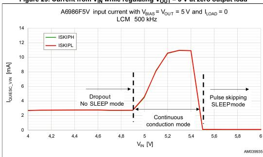
Figure 29. Current from  $V_{IN}$  while regulating  $V_{OUT} = 5 \text{ V}$  at zero output load
