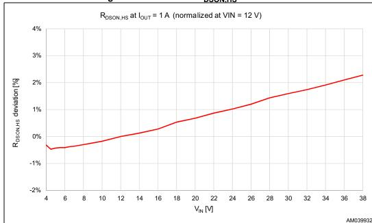
Figure 15. Normalized R<sub>DSON,HS</sub> variation
