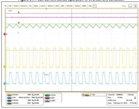
Figure 31. Peak current sense operation in overcurrent condition
