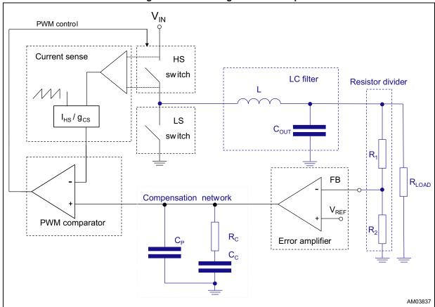
Figure 36. Block diagram of the loop
