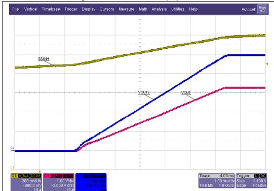
Figure 11. Ratiometric startup operation
