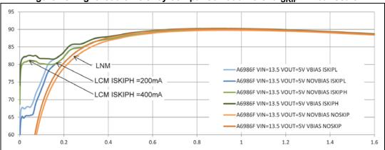
Figure 19. Light-load efficiency comparison at different I<sub>SKIP</sub> - log scale
