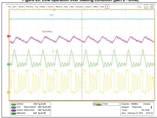
Figure 23. LCM operation over loading condition (part 2 - DCM)
