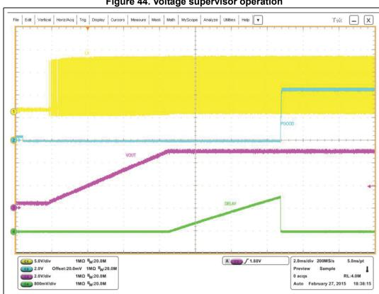
Figure 44. Voltage supervisor operation
