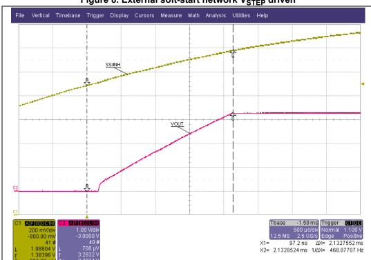
Figure 8. External soft-start network  $V_{\text{STEP}}$  driven
