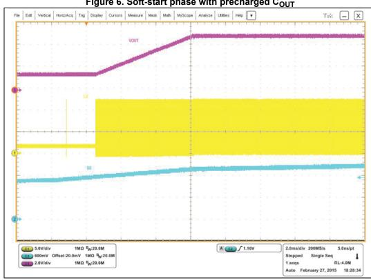
Figure 6. Soft-start phase with precharged C<sub>OUT</sub>
