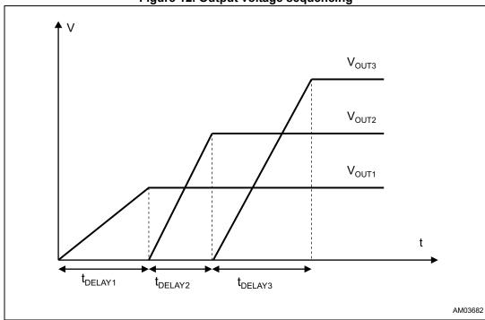
Figure 12. Output voltage sequencing
