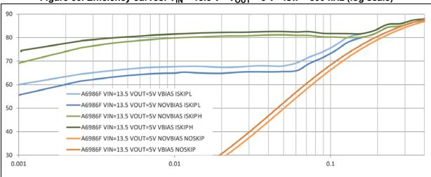
Figure 60. Efficiency curves:  $V_{IN} = 13.5 \text{ V} - V_{OUT} = 5 \text{ V} - \text{fsw} = 500 \text{ kHz}$  (log scale)
