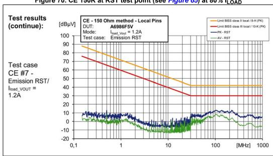
Figure 70. CE 150R at RST test point (see Figure 65) at 80% I<sub>LOAD</sub>
