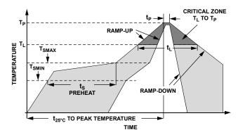
**Figure 2. Recommended Soldering Profile Limits**
