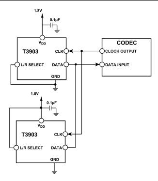
Figure 13. Stereo PDM Microphone Connection to Codec
