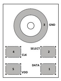
Figure 3. Pin Configuration (Top View, Terminal Side Down)
