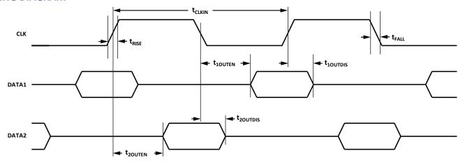
Figure 1. Pulse Density Modulated Output Timing
