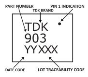
Figure 18. Package Marking Specification (Top View)
