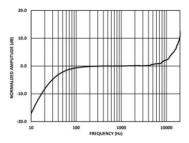
Figure 4. Typical Audio Frequency Response, High Quality Mode
