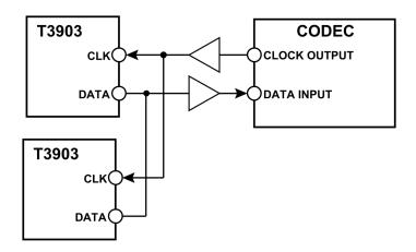
Figure 14. Buffered Connections Between Stereo T3903s and a Codec
