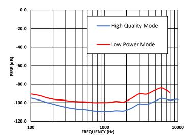
Figure 6. Power Supply Rejection (PSR) vs. Frequency
