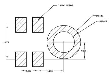
Figure 15. Recommended PCB Land Pattern Layout
