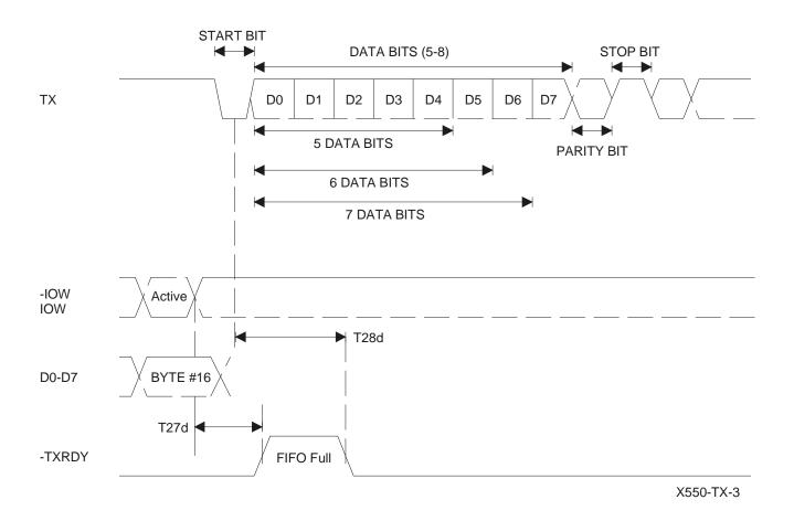
Transmit ready timing in FIFO mode
