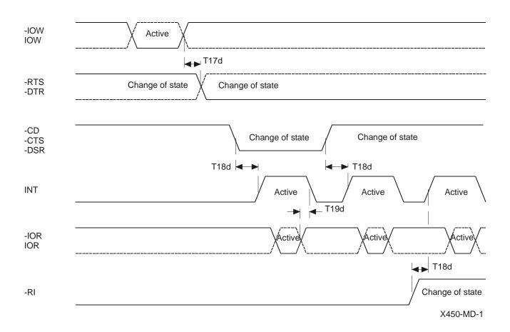
Modem input/output timing
