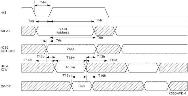
General Write Timing when using -AS signal.
