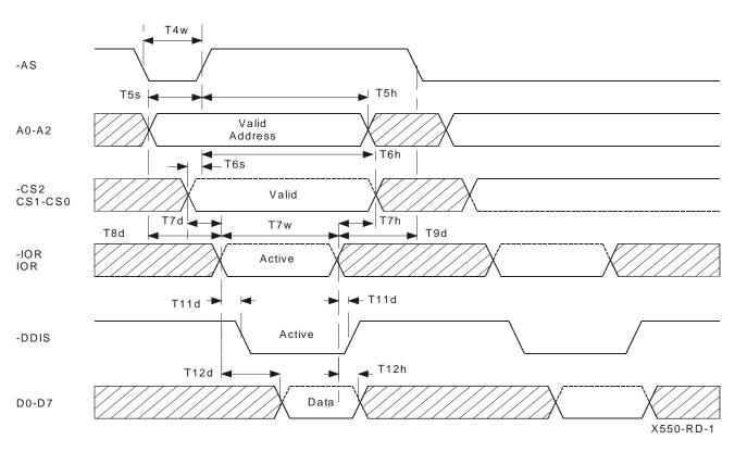
General Read Timing when using -AS signal
