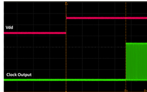
Figure 16. Startup Waveform vs. Vdd
