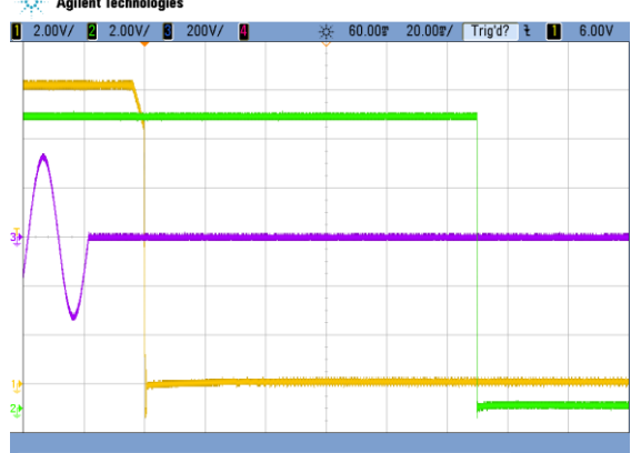
Figure 8 - Turn-On AC Line 230 VAC, full load (1 ms/div) CH1: V1 (2 V/div)
