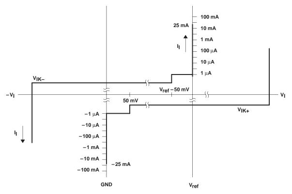
Figure 2. Tolerance Band for Clamping Circuit
