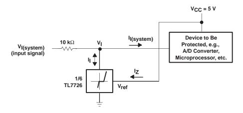
Example: If I<sub>I</sub> >> I<sub>I</sub>(system), i.e., V<sub>I</sub>(system) > V<sub>ref</sub> + 200 mV where:  $I_{I}(system) = Input \text{ current to the device being protected}$   $V_{I}(system) = Input \text{ voltage to the device being protected}$  then the maximum input voltage  $V_{I}(system) \text{max} = V_{ref} + I_{I}\text{max}(10\text{k}\Omega)$   $= 5 \text{ V} + 25 \text{ mA}(10\text{k}\Omega)$  = 5 V + 250 V = 255 V
