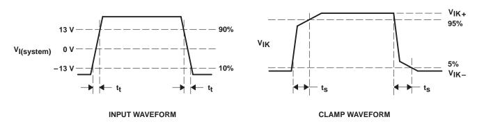
Figure 1. Switching Characteristics
