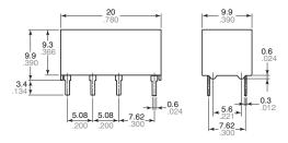
Note: External dimensions of 1 coil latching types are same as single side stable type.
