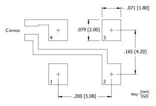
$C_{BYPASS}$  should be  $\geq 0.01$  uF.
