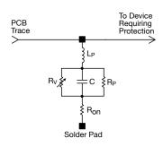
Where: = Voltage Variable resistance (per VI curve)
