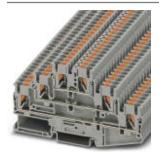
Multi-level terminal block, connection method: Push-in connection, cross section: 0.14 mm² - 4 mm², AWG: 26 - 12, width: 5.2 mm, color: gray, mounting type: NS 35/7,5, NS 35/15
