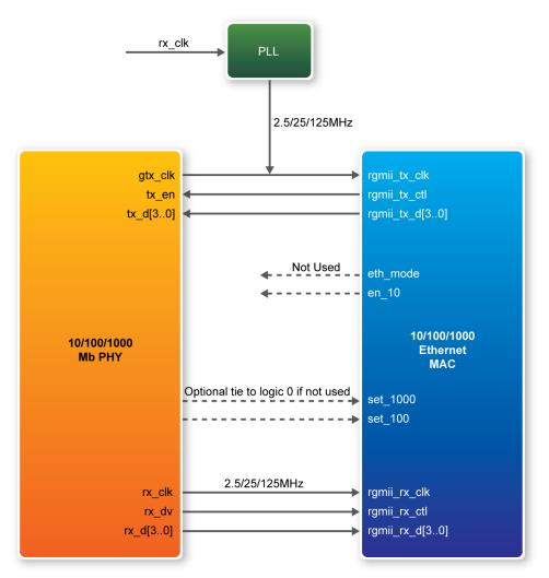
Figure 6-32 PHY connected to the MAC via RGMII
