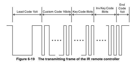
After the IR receiver on DE2-115 board receives this frame, it will directly transmit that to FPGA. In this demo, the IP of IR receiver controller is implemented in the FPGA. As **Figure 6-20** shows, it includes Code Detector, State Machine, and Shift Register. First, the IR receiver demodulates the signal inputs to Code Detector block .The Code Detector block will check the Lead Code and feedback the examination result to State Machine block.
