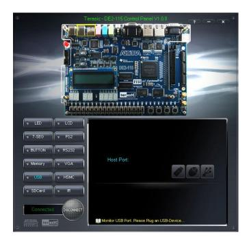
Figure 3-8 USB Mouse Monitoring Tool
