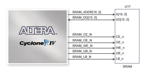
Figure 4-33 Connections between FPGA and SRAM
