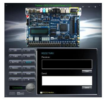
Figure 3-11 RS-232 Serial Communication
