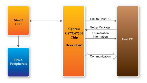
Figure 6-5 Block diagram of the USB device demonstration
