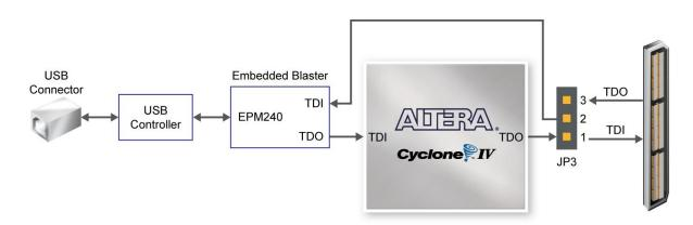
Figure 4-1 The JTAG chain on DE2-115 board
