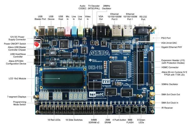
Figure 2-1 The DE2-115 board (top view)
