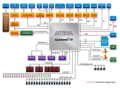
Figure 2-3 Block Diagram of DE2-115
