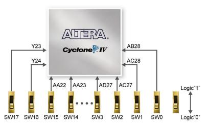
Figure 4-8 Connections between the slide switches and Cyclone IV E FPGA
