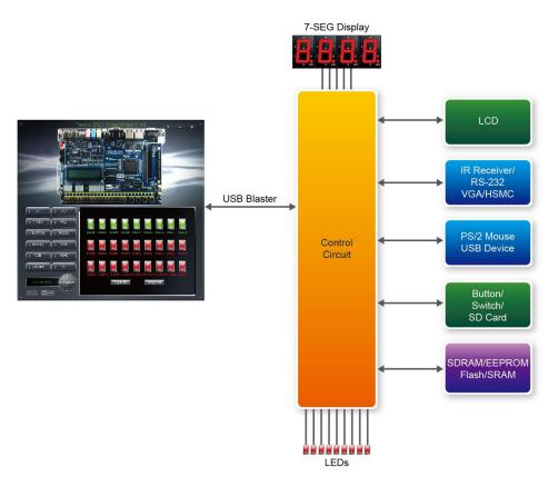
Figure 3-2 The DE2-115 Control Panel concept
