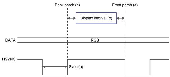
Figure 4-22 VGA horizontal timing specification
