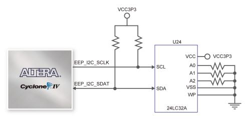
Figure 4-36 Connections between FPGA and EEPROM
