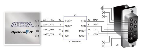
Figure 4-24 Connections between FPGA and ZT3232 (RS-232) chip
