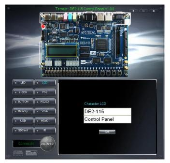
Figure 3-5 Controlling the LCD display
