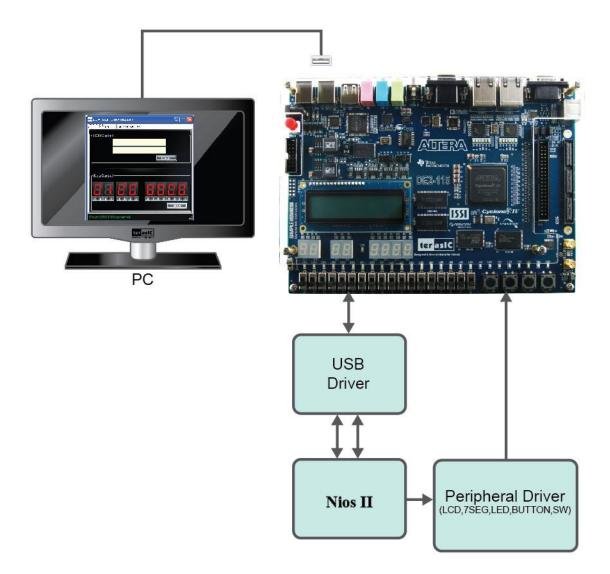
Figure 6-6 Setup for the USB device demonstration
