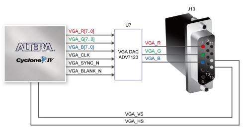
Figure 4-21 Connections between FPGA and VGA
