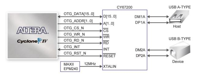
Figure 4-31 Connections between FPGA and USB (CY7C67200)
