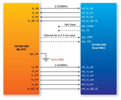
Figure 6-31 PHY connected to the MAC via MII
