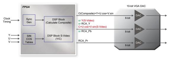
Figure 4-30 A TV Encoder that uses the Cyclone IV E FPGA and the ADV7123
