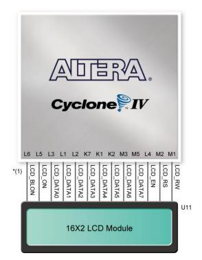
Figure 4-12 Connections between the LCD module and Cyclone IV E FPGA
