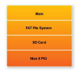
Figure 6-10 Software Stack of the SD Card Demonstration
