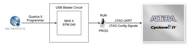
Figure 4-3 The JTAG configuration scheme
