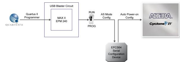
Figure 4-5 The AS configuration scheme
