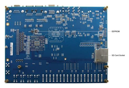
Figure 2-2 The DE2-115 board (bottom view)
