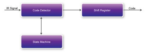
Figure 6-20 The IR Receiver controller
