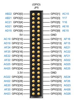
Figure 4-15 GPIO Pin Arrangement
