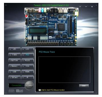
Figure 3-9 PS/2 Mouse Monitoring Tool
