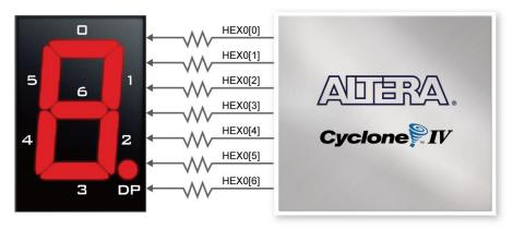
Figure 4-10 Connections between the 7-segment display HEX0 and Cyclone IV E FPGA
