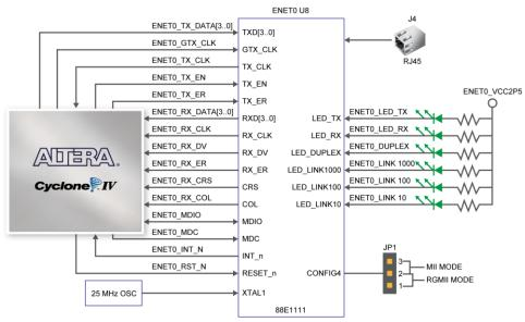
Figure 4-27 Connections between FPGA and Ethernet
