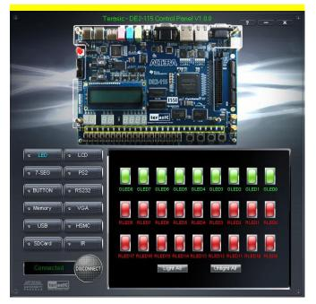
Figure 3-3 Controlling LEDs
