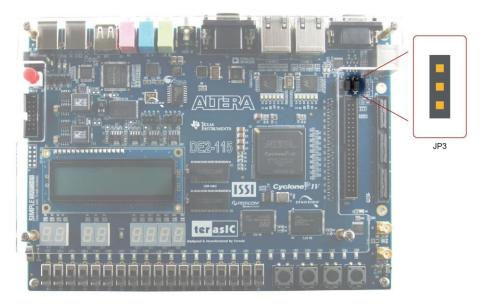
Figure 4-2 The JTAG chain configuration header
