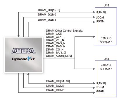
Figure 4-34 Connections between FPGA and SDRAM
