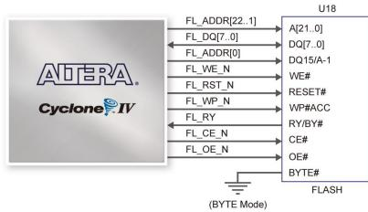
Figure 4-35 Connections between FPGA and Flash
