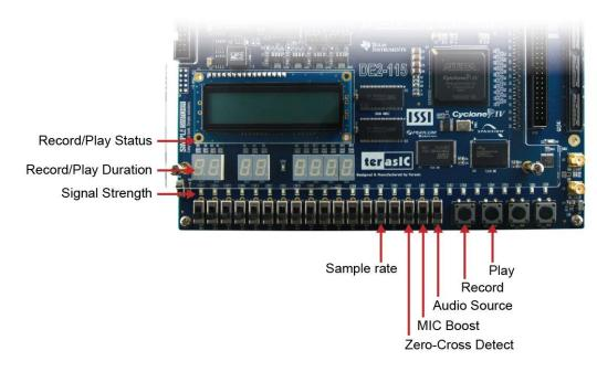
Figure 6-25 Man-Machine Interface of Audio Recorder and Player
