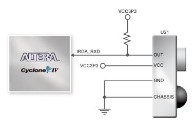
Figure 4-32 Connection between FPGA and IR
