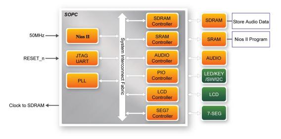
Figure 6-26 Block diagram of the audio recorder and player
