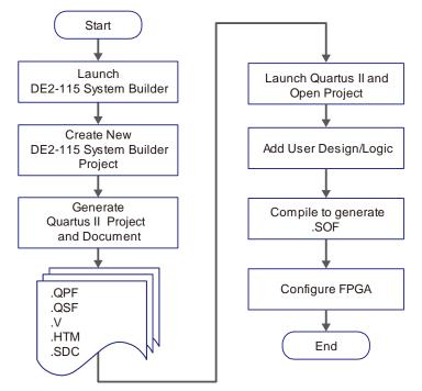
Figure 5-1 The general design flow of building a design
