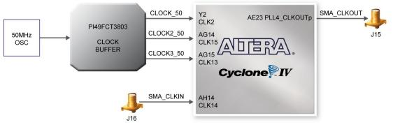
Figure 4-11 Block diagram of the clock distribution
