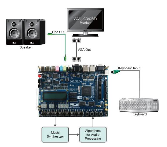
Figure 6-24 The Setup of the Music Synthesizer Demonstration
