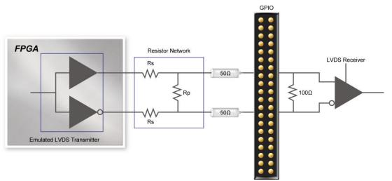
Figure 4-19 Using Emulated LVDS on GPIO
